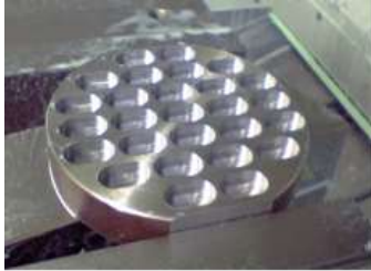
Pocket Size : 9 \times 15 \times Depth 4 mm
