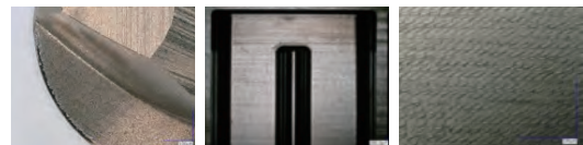
Near the tip After 360 min milling Whole milling surface Enlarged milling surface
