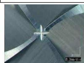
Smooth chip evacuation reduces damage at the tip.
