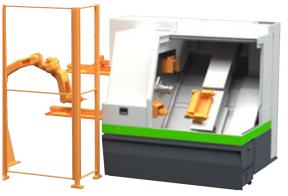
Feeding from a robot via a loading shuttle
