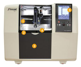
To produce narrow tolerance parts, the micro abrasive waterjet cutting system must also be accompanied by a very precise motion capability that accurately reproduces the programmed geometry. The Finecut machine have been designed to optimise the part precision to a new level.
