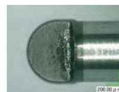
Tool after 45h of milling
