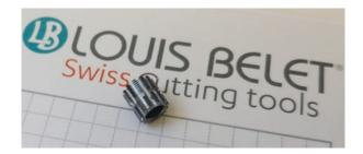
Tested at several customers in production, this hobbing technique makes it possible to machine small modules in multiple materials without burrs.
