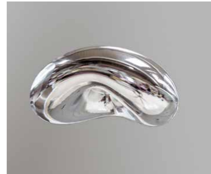
"The bean" was not polished but only milled on KERN Micro with this reflective surface
